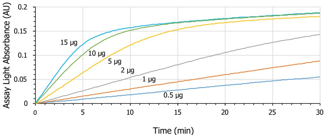
**Figure 1.** Effect of BirA quantity on reaction rate (constant volume and substrate quantity).
